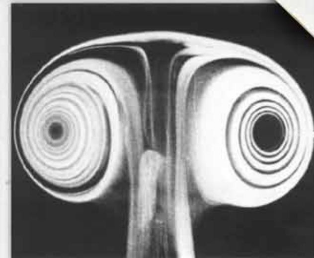
Photo showing a fundamentally new and highly efficient way of fire suppression for oil and gas fountains that arise from accidents on the wells. The fire is suppressed through a pulse impact of an air vortex ring filled with dispersed extinguishing powder
