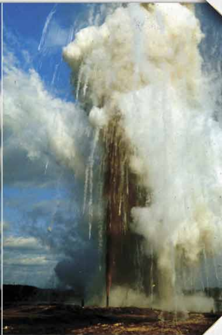
Photo showing a fundamentally new and highly efficient way of fire suppression for oil and gas fountains that arise from accidents on the wells. The fire is suppressed through a pulse impact of an air vortex ring filled with dispersed extinguishing powder
